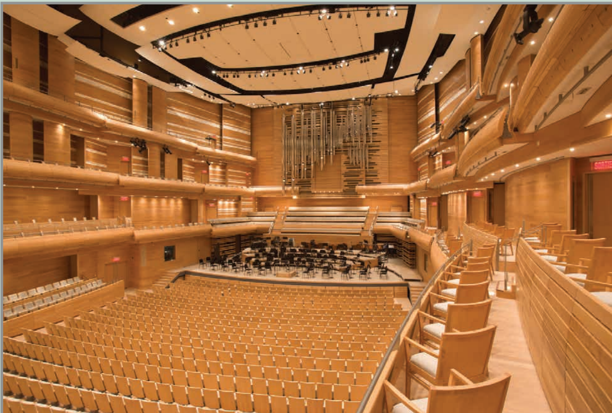
The auditorium is a classic shoebox design, in that "it's narrow and tall, but it's not a box—it's curvilinear," said Diamond, referring to the striking convex arcs and gently sweeping curves that characterize the walls, balcony fronts, and boxes.
